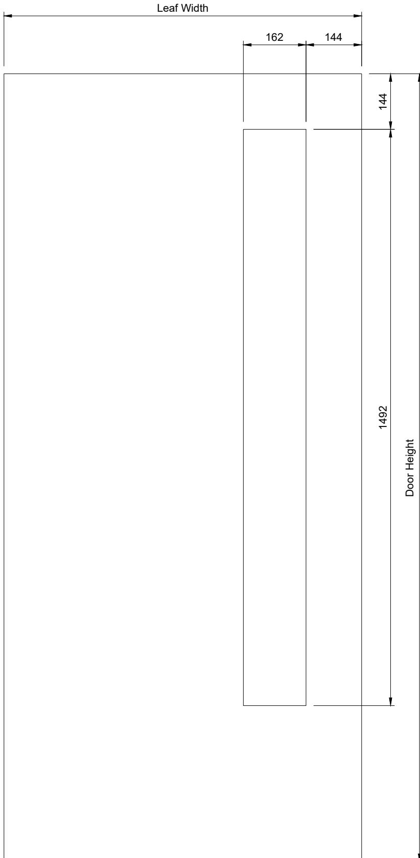
Size Given Is The **Machined** Aperture Size In The Door
